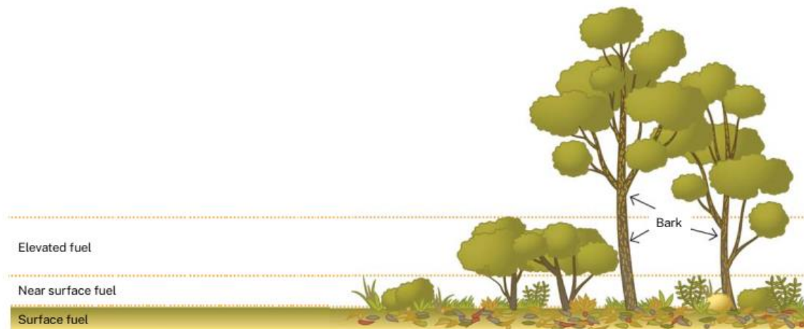
Figure 7: Categories of fuel along the vertical plane from the Bushfire Centre of Excellence and the Department of Fire and Emergency Services WA (2021). Note that the canopy fuel is not labelled however it is the uppermost layer in the diagram.
