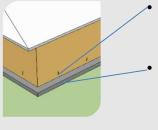
Inadequate ventilation of wall cavities can lead to deterioration and mould growth; however, gap openings more than 1.8mm can allow ember entry. A concrete slab on ground is preferred for bushfire, while for flooding a raised slab is preferred.
